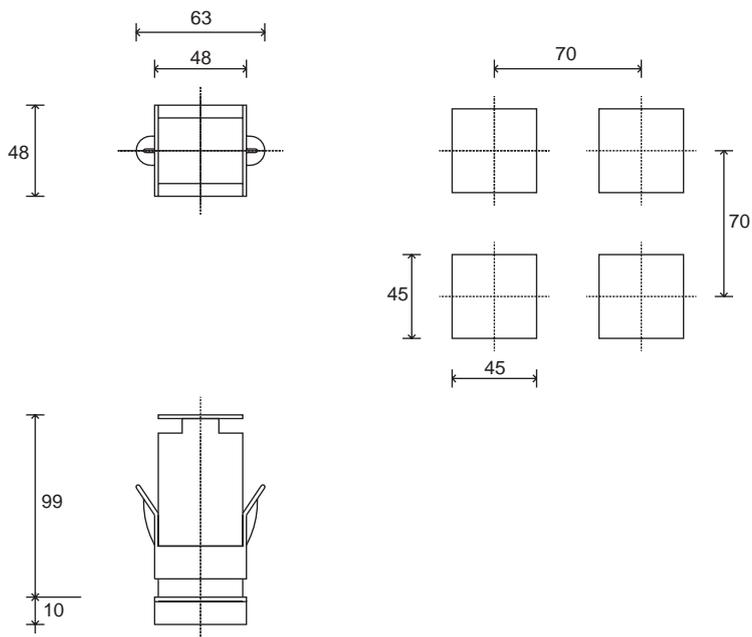
Face avant: 48x48mm (1/16DIN). Profondeur 99mm
